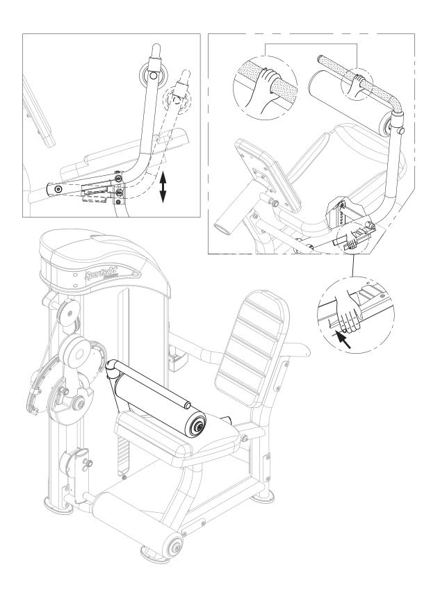
\* To move the seat back position toward yourself, simply pull it. To move the seat back away from yourself, pull the knob and press the seat back.
