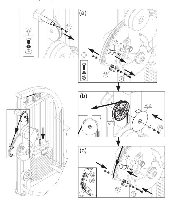
(d). After completing the cable installation, hold the upper stack carriage set (22), and then take out the stack fork (A7). Gently lower the upper stack carriage set (22). (Note: Please make sure that the cable is running in the grove of the pulley. Rotate the CAM to check for cable interference and its tightness. If the cable is too loose or too tight, follow the cable adjusting instruction to adjust it.)
