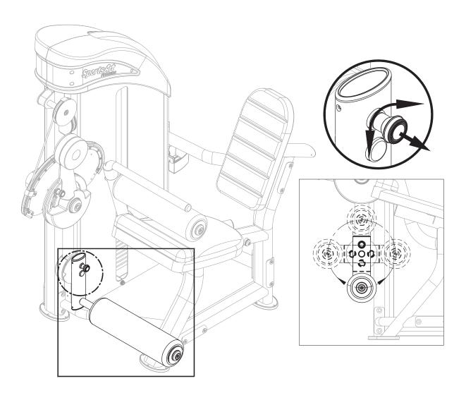
\* Pull out the knob on the rotator arm of CAM. Place the rotator as desired for use. When released, the knob automatically engages to secure the position.
