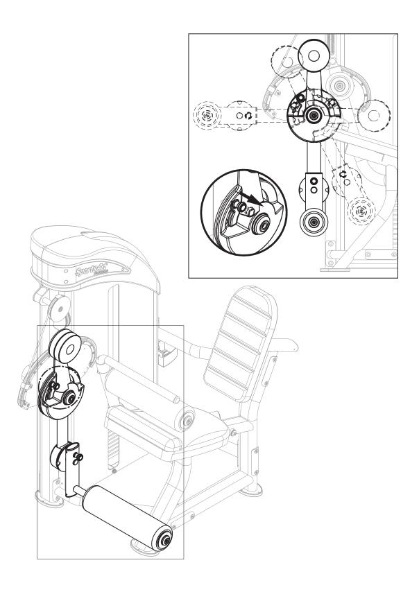
\* With your left hand on the handle and your right hand on the release lever, adjust the cushion height.
