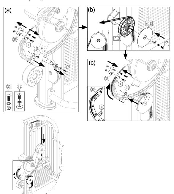
(d). After completing the cable installation, hold the upper stack carriage set (22), and then take out the stack fork (A7). Gently lower the upper stack carriage set (22). (Note: Please make sure that the cable is running in the grove of the pulley. Rotate the CAM to check for cable interference and its tightness. If the cable is too loose or too tight, follow the cable adjusting instruction to adjust it.)
