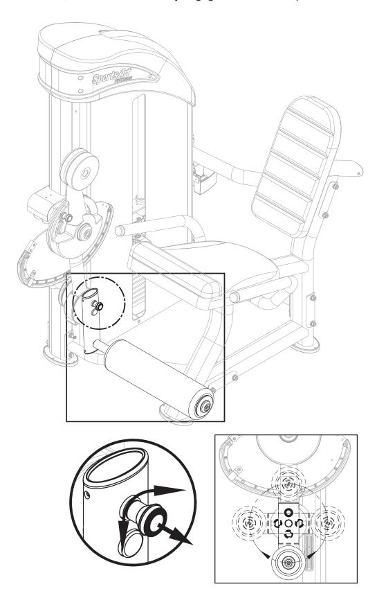
\*Pull out the knob on the rotator arm of CAM. Place the rotator as desired for use. When released, the knob automatically engages to secure the position.
