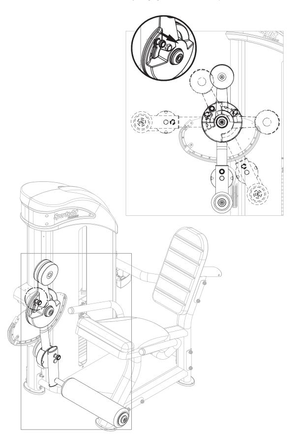
\* To move the seat back position toward yourself, simply pull it. To move the seat back away from yourself, pull the knob and press the seat back.
