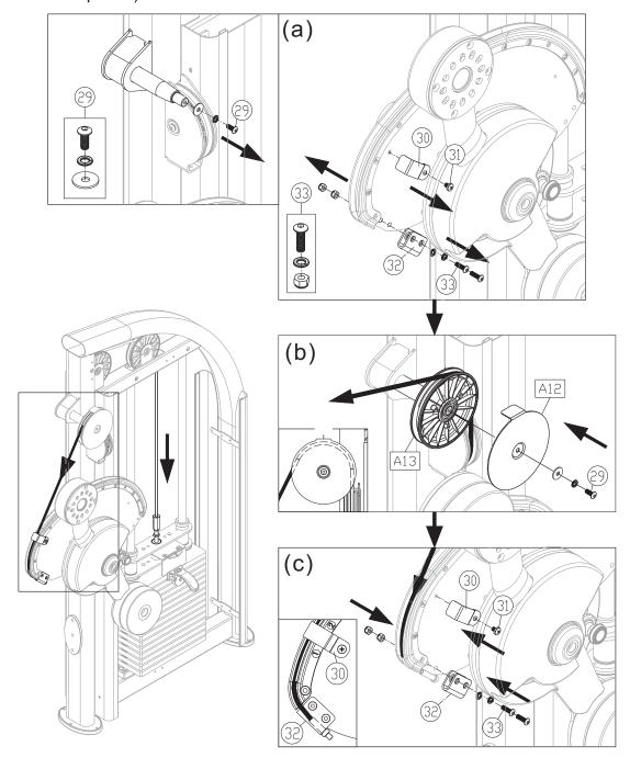
(d). After completing the cable installation, hold the upper stack carriage set (20), and then take out the stack fork (A7). Gently lower the upper stack carriage set (20). (Note: Please make sure that the cable is running in the grove of the pulley. Rotate the CAM to check for cable interference and its tightness. If the cable is too loose or too tight, follow the cable adjusting instruction to adjust it.)
