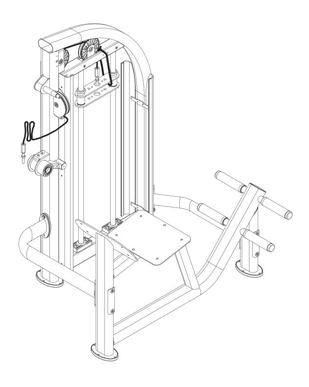
\*Loosen and remove the screws (21) (22) and the connecting plates from the connectors (A3) (A27) (A28) as shown. Carefully set each piece aside.
