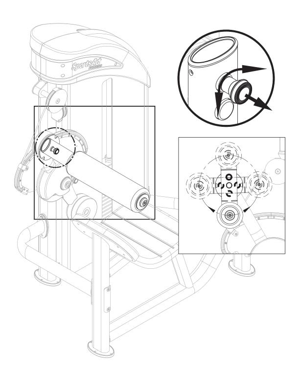
\* Pull out the knob on the rotator arm of CAM. Place the rotator as desired for use. When released, the knob automatically engages to secure the position.
