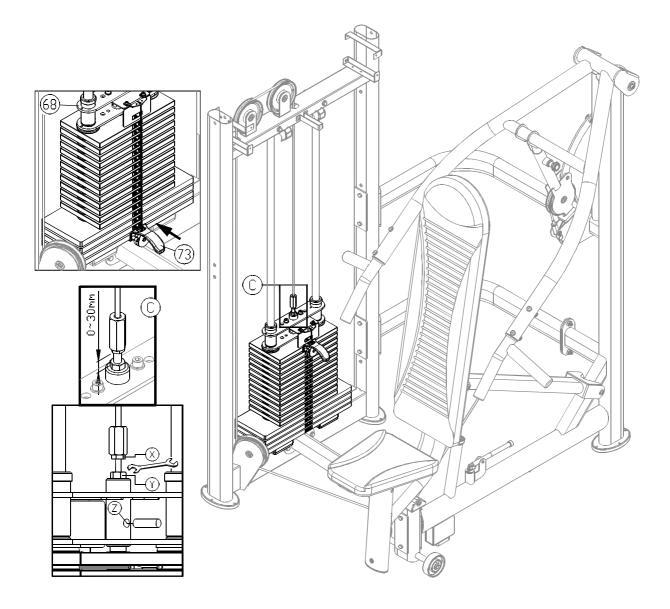
Insert the stack fork into the gap under the lowest weight plate. Then adjust the large nut at area D. Adjust until the upper stack carriage moves slightly. To adjust the cable, first insert an open end wrench into (Z) hole. Loosen (Y) nut. Then adjust (X) nut. If the cable is too long, adjust (X) nut downward. If too short, adjust (X) nut upward. After adjusting (X) nut, tighten (Y) nut against the weight stack to secure this position.
