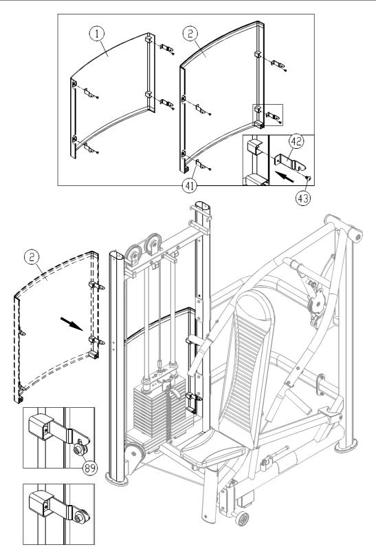
12-1. Before installing the upper and lower rear covers, first separate A and B (41,42) set brackets by side.
