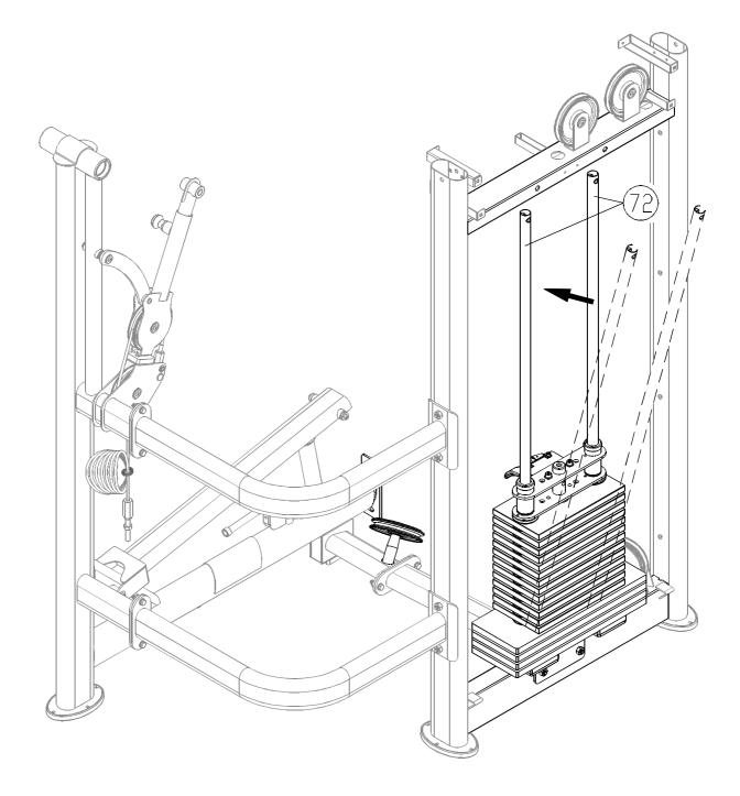
2-7. Tilt the guide rods (72) back into place.
