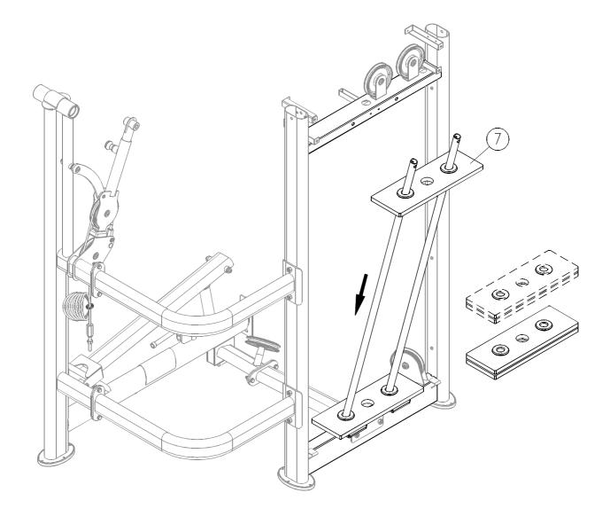
2-4. Insert and lower the four large (7.5 kg) weight plates into place on the guide rods one at a time (7). NOTE: The convex side faces up.
