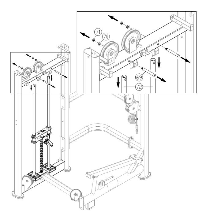
2-2. Remove hardware (69,70,71). Guide the guide rods (72) downward as shown.
