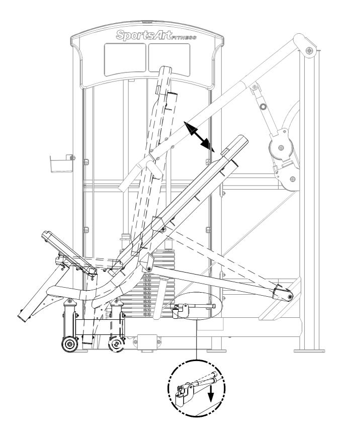
To adjust the seat back position, press the adjustment lever with your foot. Then move the seat back to the position you desire.
