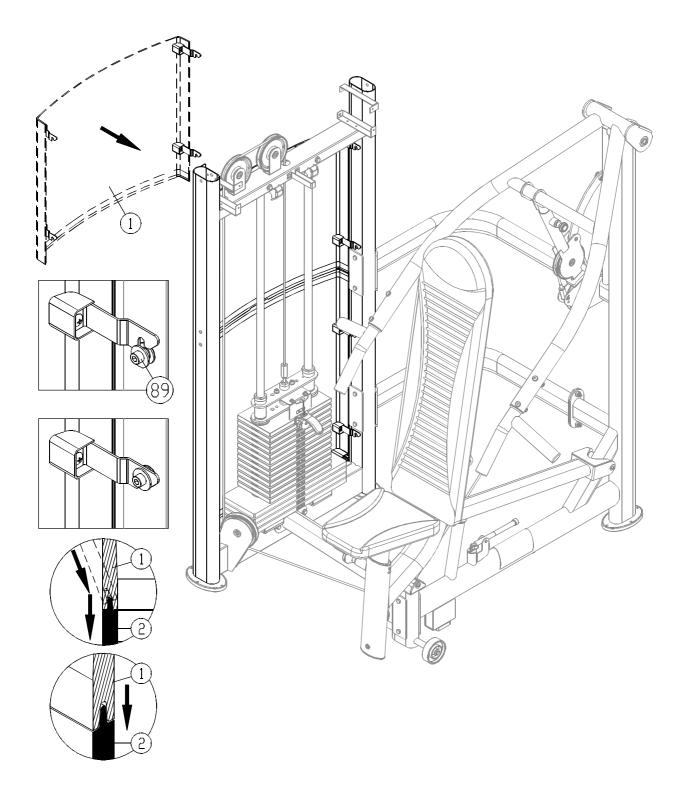
12-3. Hang back cover A (1) onto screws (89). Simultaneously, hook back cover A (1) into back cover (2).
