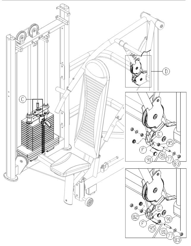
If there is no way to adjust area C, please rotate area C out 30mm (about 1 inch). Remove the bushing (95), axle (81), washer (77), nut (83), and soft cap (91) from hole E in area D. Put the cable screw (82) in hole F. Then put the bushing (95), axle (81), washer (77), nut (83), and soft cap (91) back in place. Then secure the cable as in step (9) as shown.
