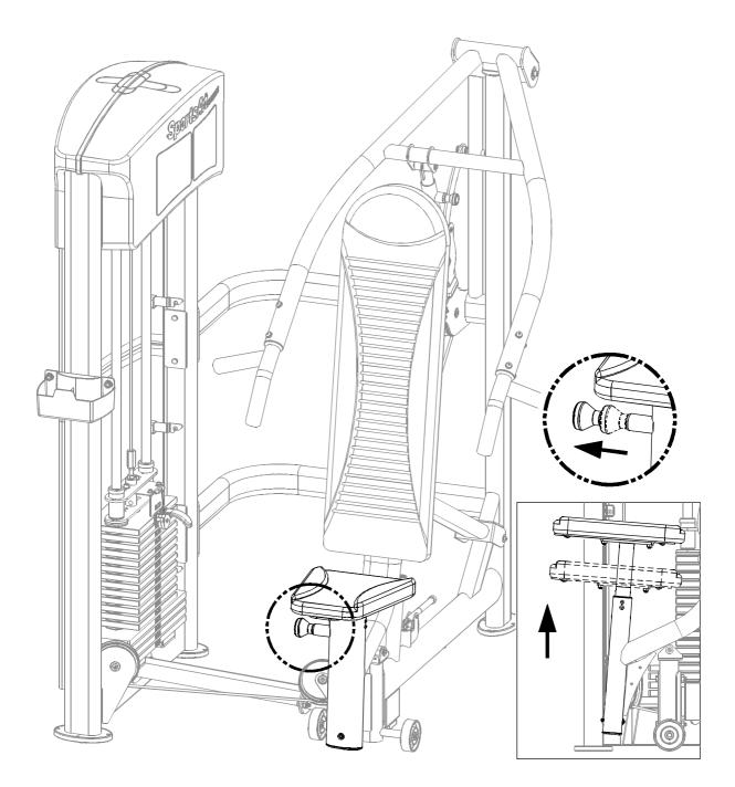
To raise the seat bottom, simply pull it upward. To lower the seat bottom, pull the adjustment knob outward and lower the seat bottom.
