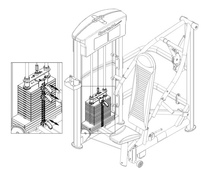
16-1. Insert the stack fork to make sure that every weight plate can be engaged easily.
