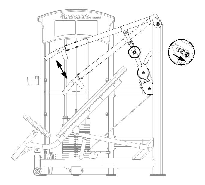
To adjust the press handle, pull the adjustment knob outward and move the handle to the desired position.
