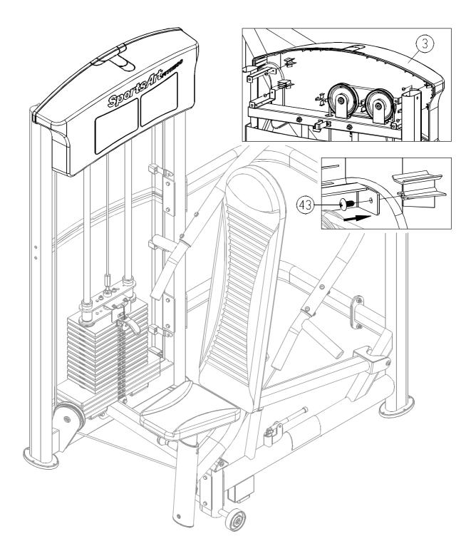
13-1. Use screws (43) to secure the front top cover onto the stack tower.
