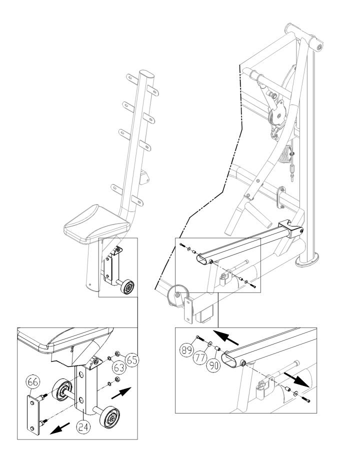
5-1. First, remove the sleeve (90) and hardware (77,89). Then remove hardware (63,65) from the seat frame (24) and connector (66). Set aside these parts for use in the next step.
