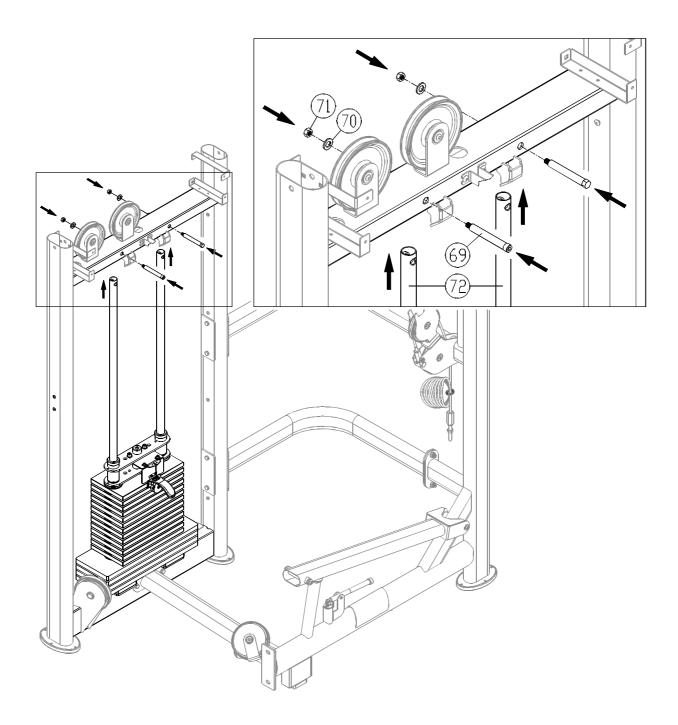
2-8. Lift the guide rods (72) up into their mounting station. Then secure them with hardware (69,70,71).
