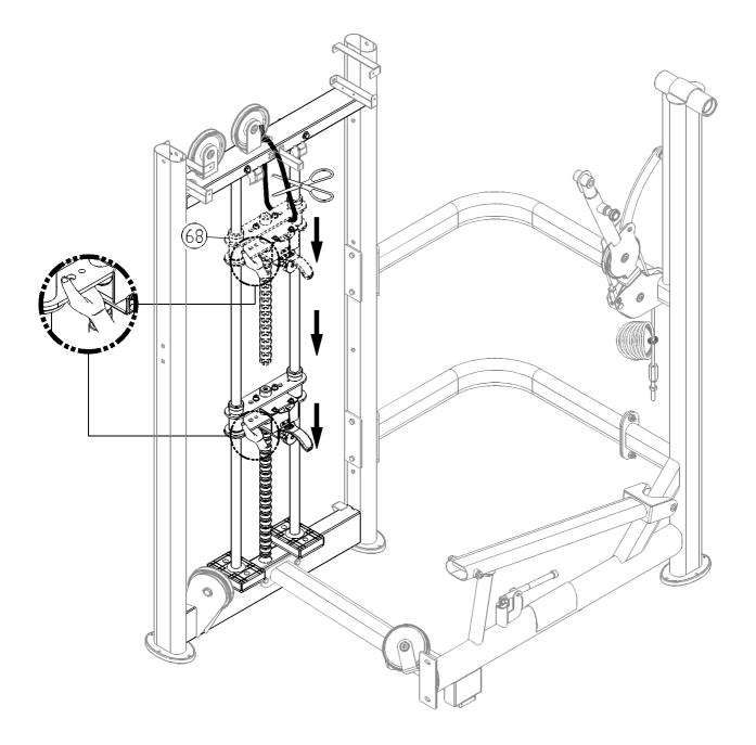
2-1. Hold upper stack carriage (68) and cut the zip tie. Gently lower the upper stack carriage (68) into place as shown.
