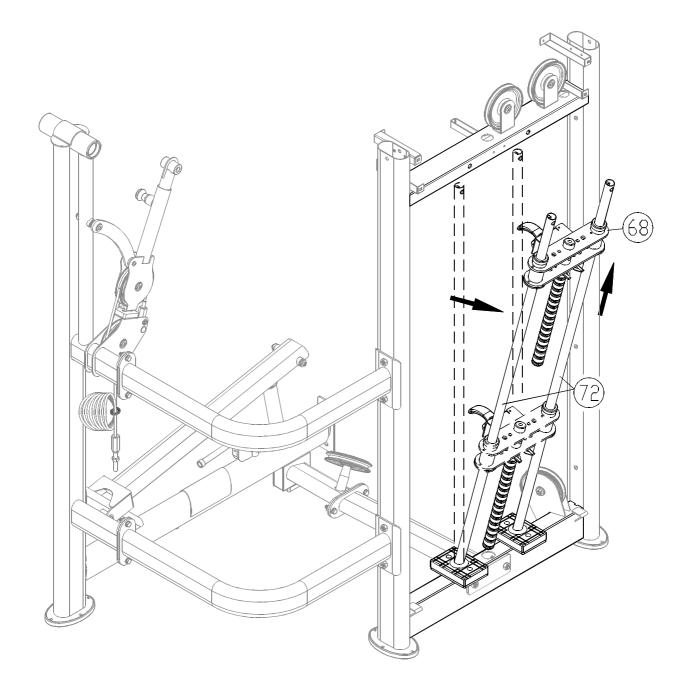
2-3. Tilt the guide rods (72) backward. Then lift the upper stack carriage (68) off the guide rods as shown. Carefully set the upper stack carriage aside.
