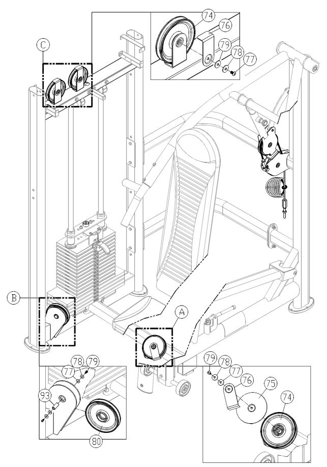
9-1. Before installing the cable, first remove the cover (75,76,77,78,79) in area A and the pulley wheel (77,78,79,80,93) in area B and cover plate (76,77,78,79) in area C as shown. Note: Keep pulley wheel A (74) on the product. Set hardware aside in a safe place for later use.
