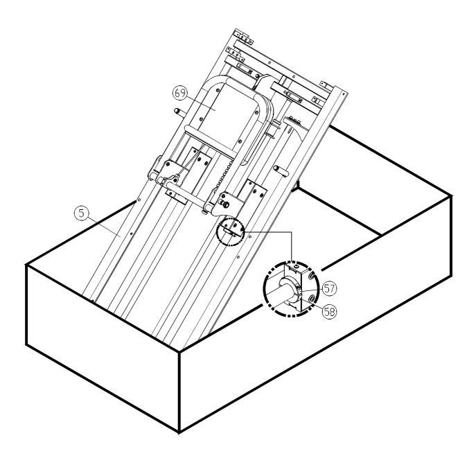
Before tilting up the main frame (5), make sure that set rings A,B (57,58) are in place. Otherwise, the knee platform (69) can slide downward. After preventing the knee platform (69) from sliding, tilt the main frame (5) upward as shown.
