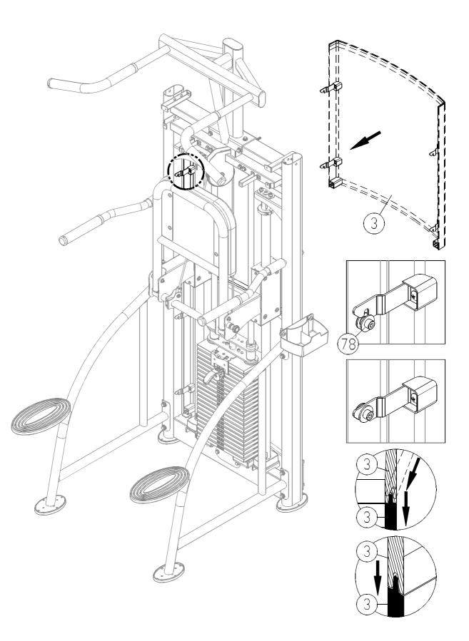
7-3. Hang upper back cover (3) onto screws (78). Simultaneously, hook upper rear cover (3) into cower rear cover (3).
