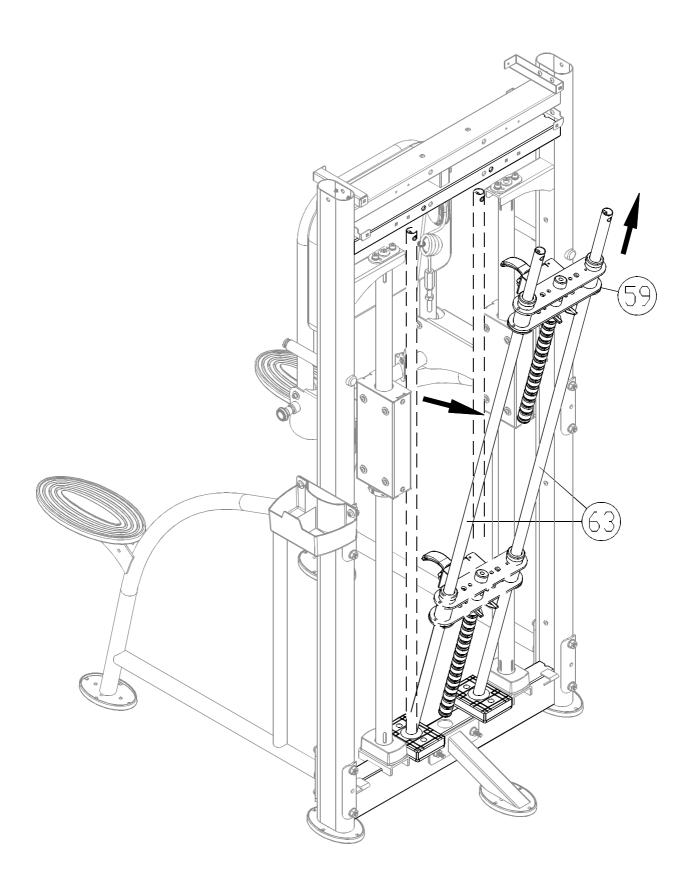
2-3. Tilt the guide rods (63) backward as shown. Then lift the upper stack carriage set (59) from the guide rods as shown. Carefully set the upper stack carriage set aside.
