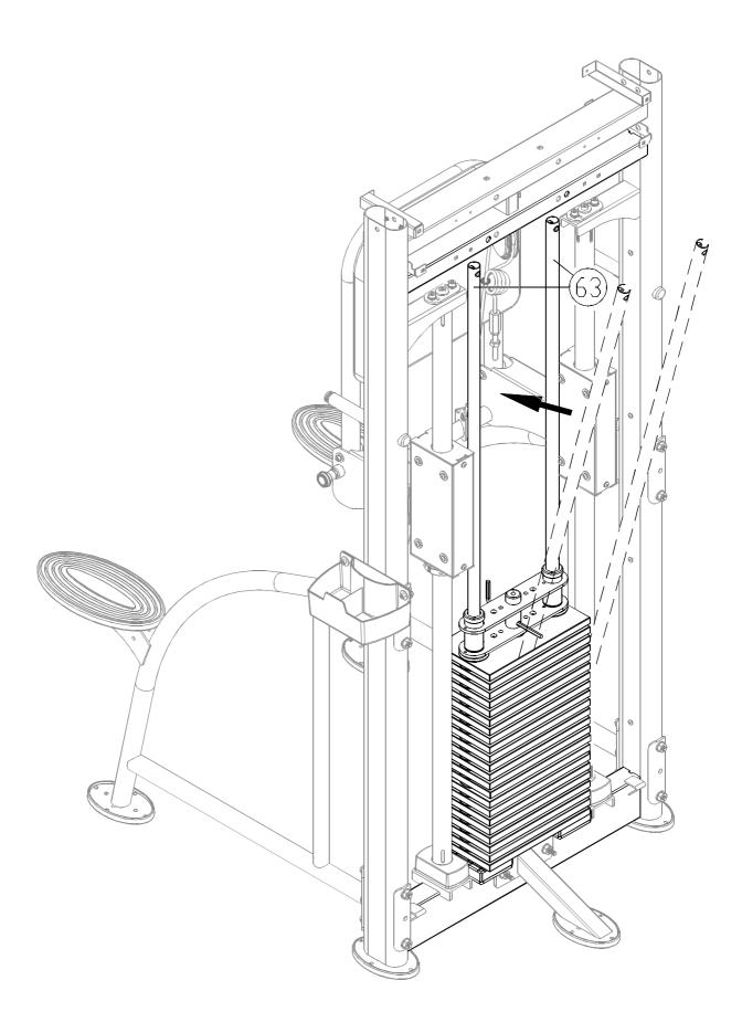
2-7. Tilt the guide rods (63) back into place.
