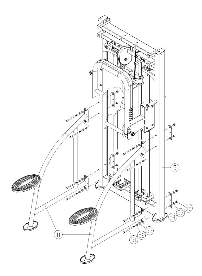
1-1. Connect the front support (11) to the main frame (5). Attach connector (54) with hardware (51,52,53,55) but do not fully tighten bolts.
