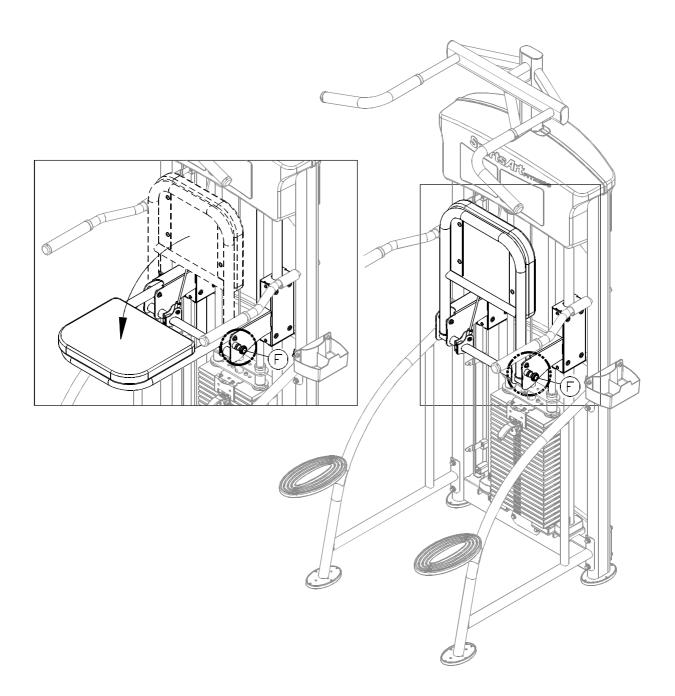
To change the knee platform position, pull out knob F. The knee platform can be placed up, out of the way, or down, in place to assist you.
