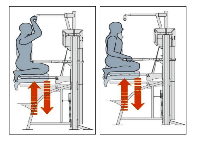
Please see operating instructions on the product. Exercise as instructed to test unit operation. Insert the stack fork at the heaviest weight setting at which you can safely operate the equipment. Exercise to lift the stack several times. Then inspect the cable for proper tightness. If necessary, make adjustments according to the instructions in this manual.
