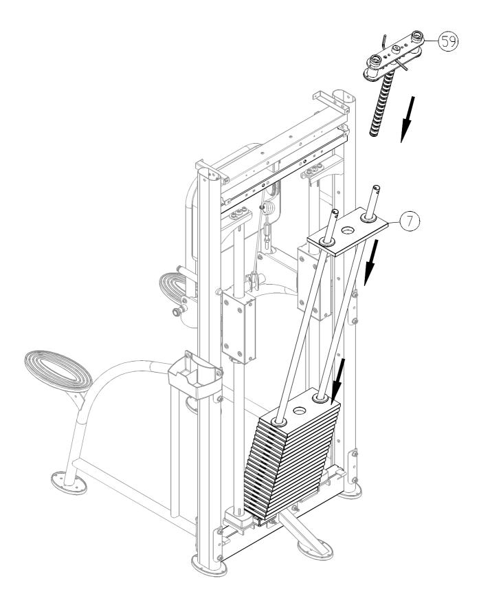
2-5. Insert and lower the 22 5KG weight plates (7) into place on the guide rods as shown.
