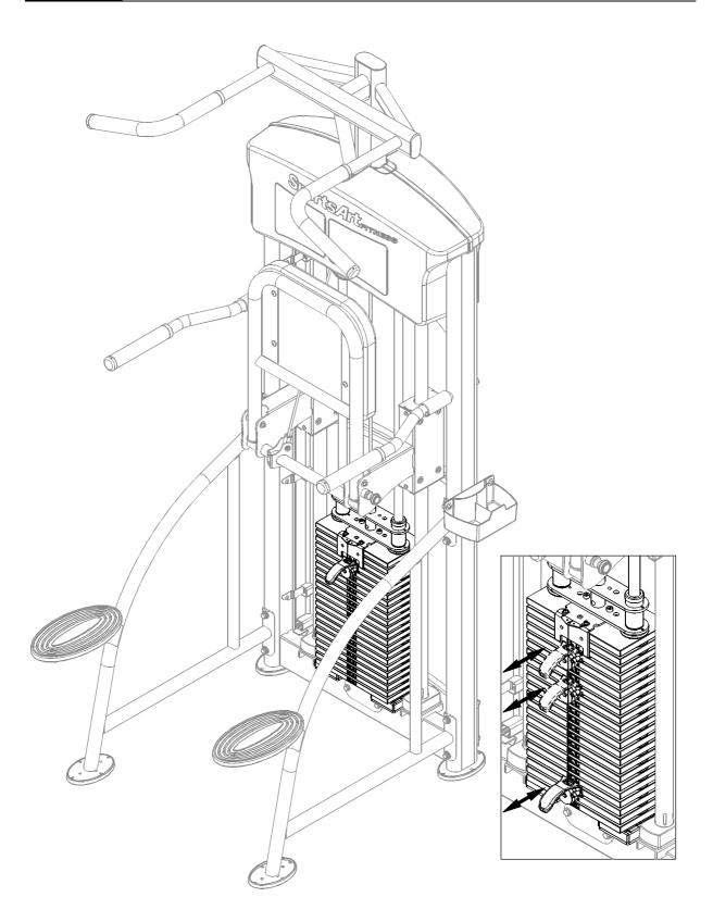
10-1. Insert the stack fork to make sure that every weight plate can be engaged easily.
