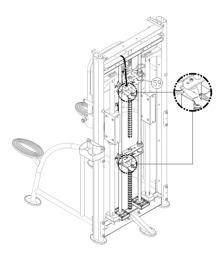
2-1. Hold the upper stack carriage set (59). Then cut the zip tie that holds it in place. Gently lower the upper stack carriage set (59) into place as shown.
