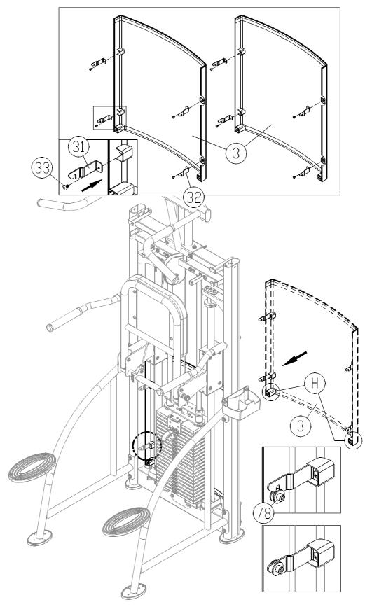
7-1. First, identify left and right side back cover brackets A, B (31,32). Then use hardware (33) to secure back cover brackets onto stack cover (3) left and right sides as shown.7-2. Then hook the stack cover (3) onto the screw (78).
