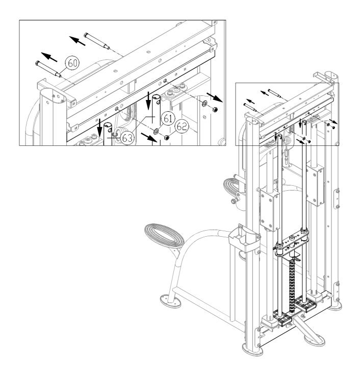
2-2. Remove hardware (60,61,62). Then guide the guide rods (63) downward as shown.
