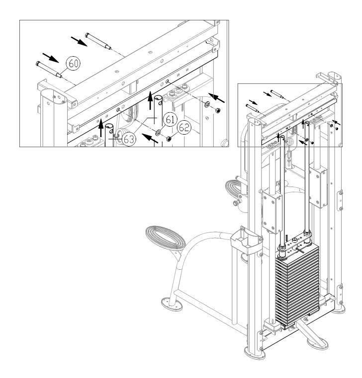
2-8. Lift the guide rods (63) up into their mounting station. Then secure them with hardware (60,61,62).
