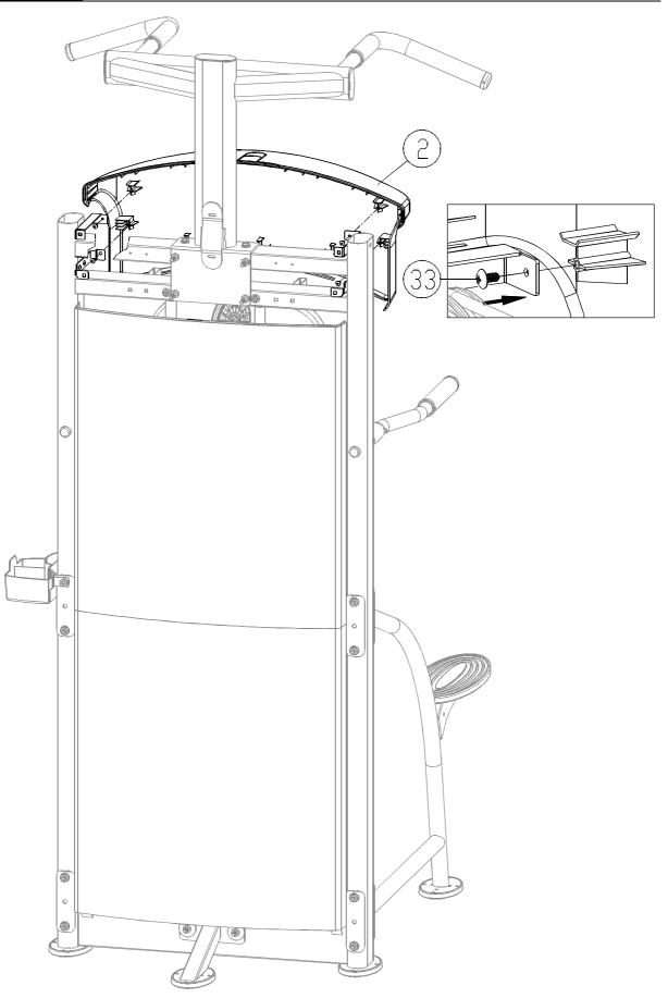
8-1. Use screws (33) to secure the front top cover (2) onto the frame as shown.
