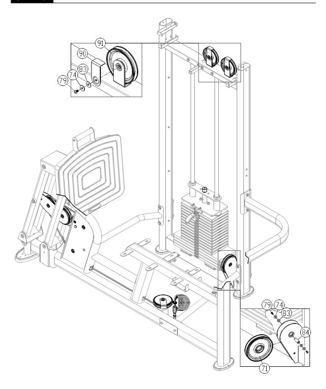
5-1. First, remove hardware (74,79,84,83) from pulley A(71), and cover (90,74,79,83) from pulley B(91).
