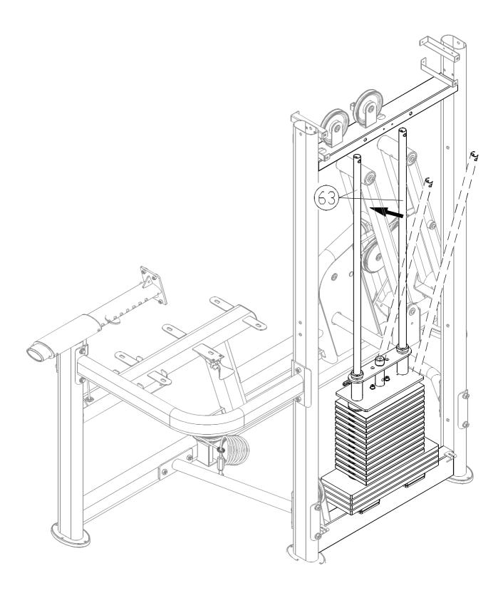
2-7. Push the guide rods (63) back into place.
