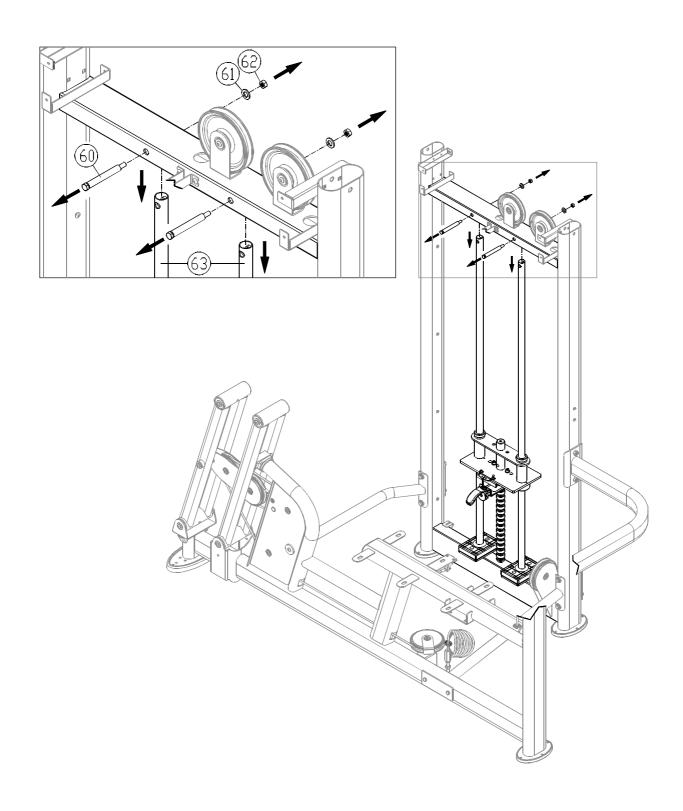
2-2. Remove hardware (60,61,62). Then lower the guide rods (63) as shown.
