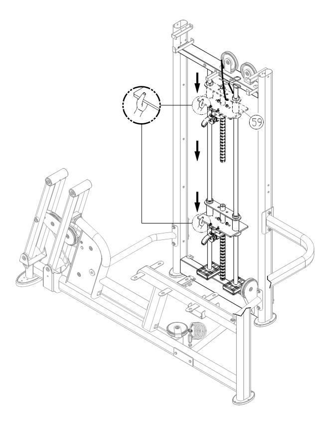
2-1. Hold the upper stack carriage (59). Then cut the zip tie. Gently lower the upper stack carriage (59) into place as shown.
