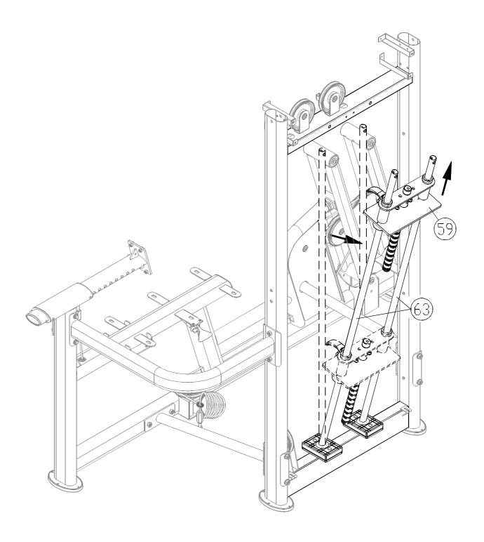
2-3. Tilt the guide rods backward (63). Then remove the upper stack carriage (59) from the guide rods as shown. Carefully set aside the upper stack carriage.
