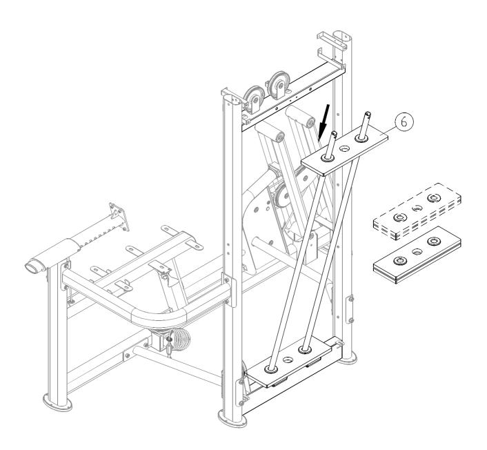
2-4. First, gently insert the four large (7.5kg) weight plates (6) into place one-by-one on the guide rods.
