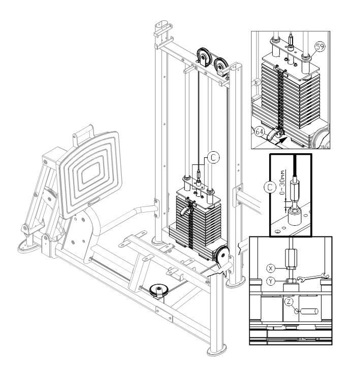
Insert the stack fork into the gap under the lowest weight plate. Then adjust the large nut at area C. Adjust until the upper stack carriage moves slightly.
