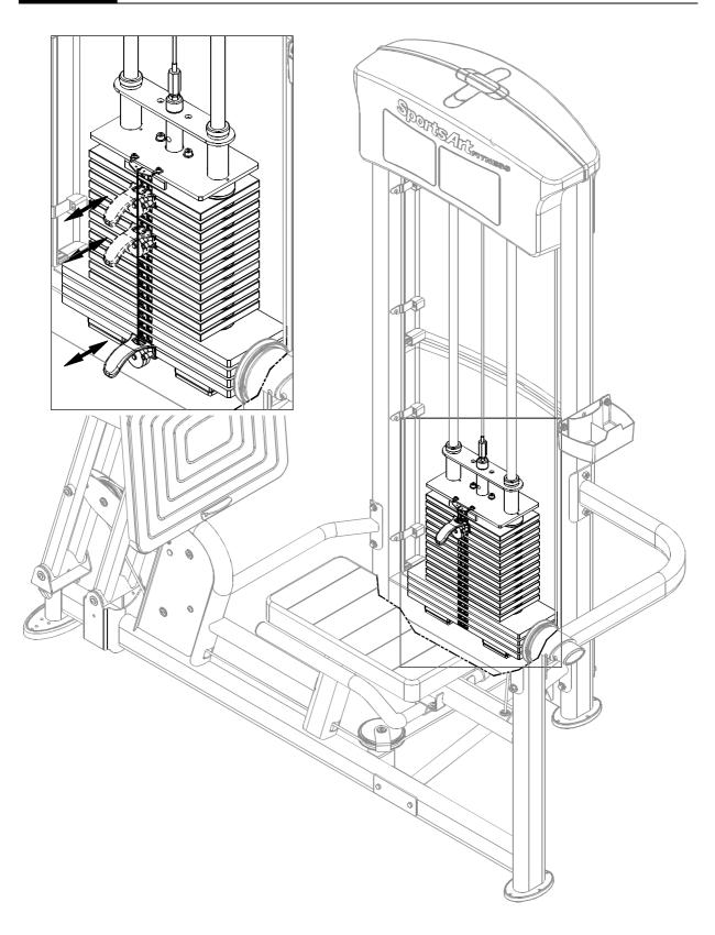
15-1. Insert the stack fork to make sure that every weight plate can be engaged easily.
