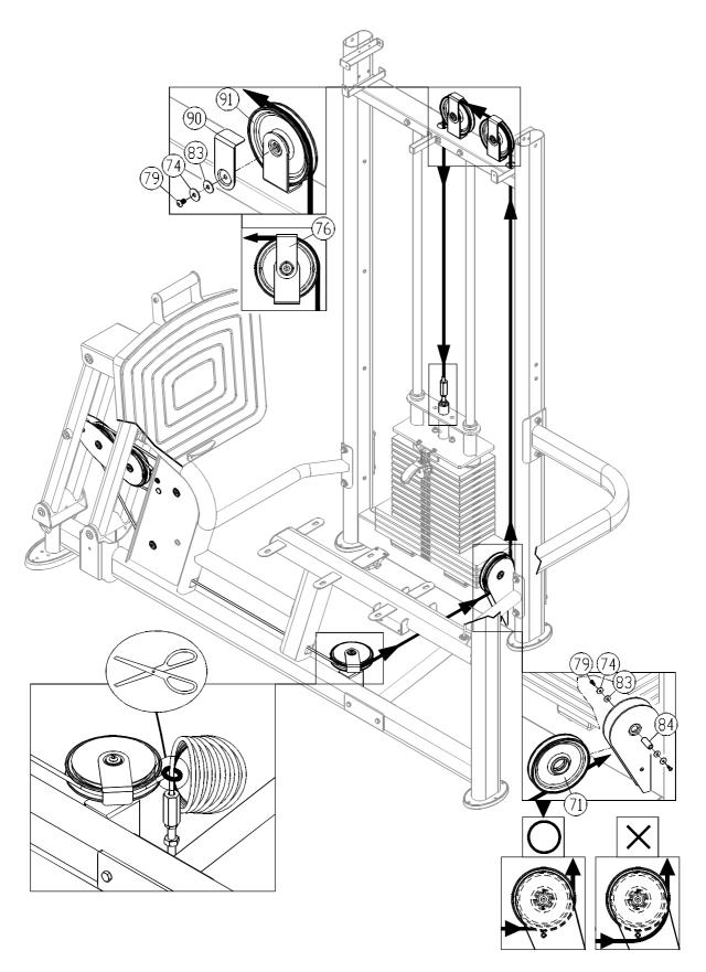
5-2. First, cut the zip tie. Thread the cable onto pulley A (71). Then secure the pulley with hardware (74,79,84,83).
