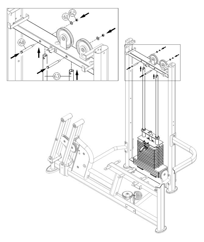
2-8. Lift the guide rods (63) up into their mounting stations. Then secure them with hardware (60,61,62)
