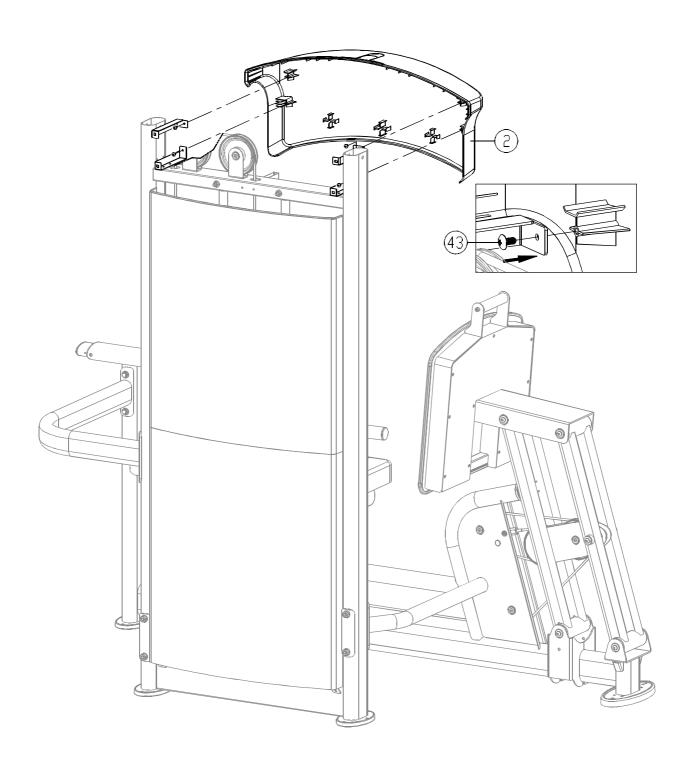
12-1. Use screws (43) to secure the front top cover (2)onto the stack tower.
