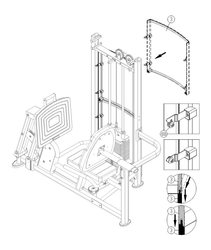
11-3. Hang back cover (3) onto screws (88). Simultaneously, hook back cover (3) into rear cover (3).
