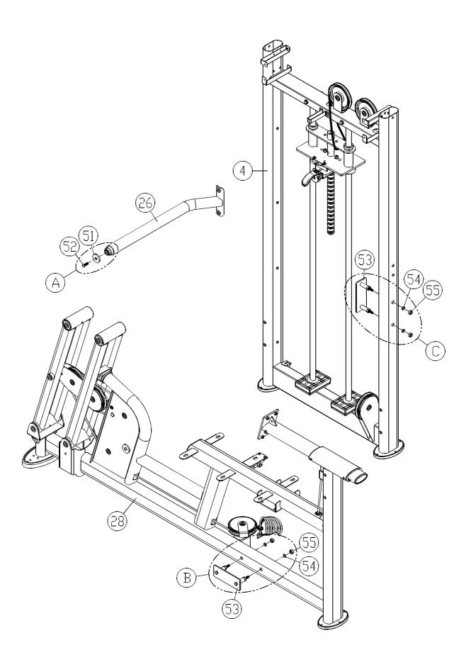
1-1. First, remove connector plates (53) from areas A,B,C by removing screws (51,52) and nuts (54,55). Set these parts aside for later use.
