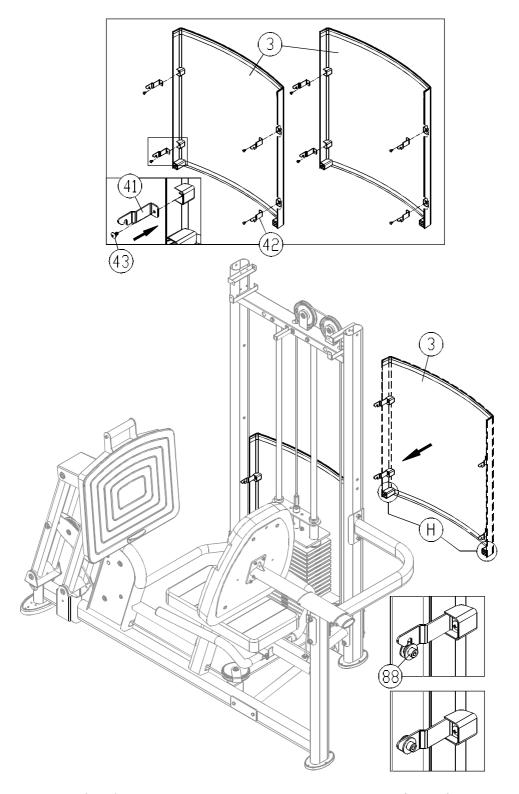
11-1. First, identify left and right side rear cover brackets A, B (41,42). Then use hardware (43) to secure rear cover brackets onto cover (3) left and right sides as shown.
