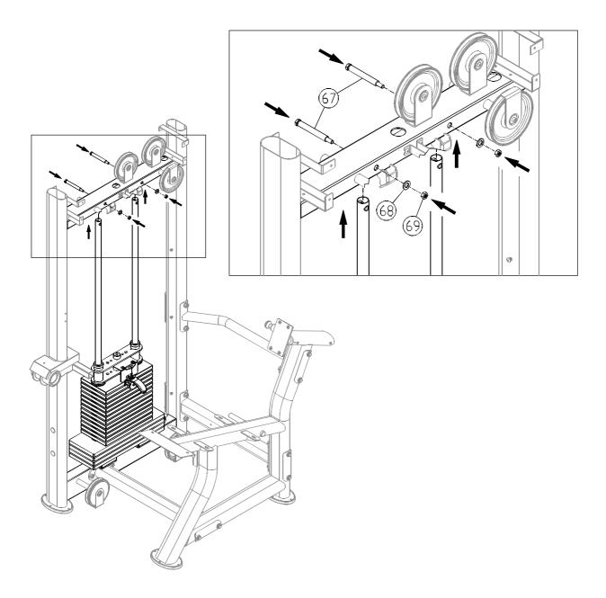
2-8. Lift the guide rods (70) up into their mounting station. Then secure them with hardware (67, 68, and 69).
