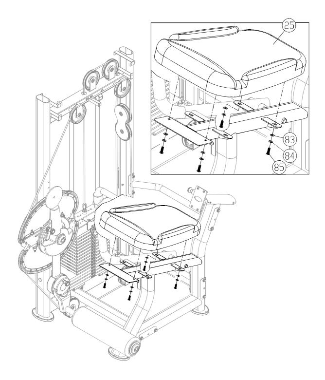
9-2. Use hardware (83,84,85) to secure the seat bottom (25) in place as shown.
