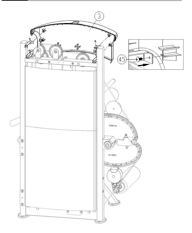
12-1. Use screws (45) to secure the front top cover (3) in place on the main frame as shown.
