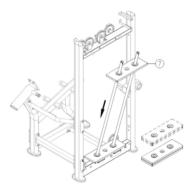
2-4. Insert and lower the four large (7.5 kg) weight plates (7) into place on the guide rods one at a time.
