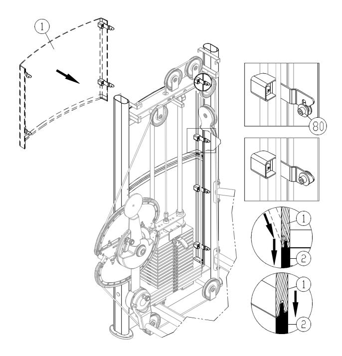
11-3. Hang upper rear cover (1) onto screws (80). Simultaneously, hook upper rear cover (1) into lower rear cover (2).
