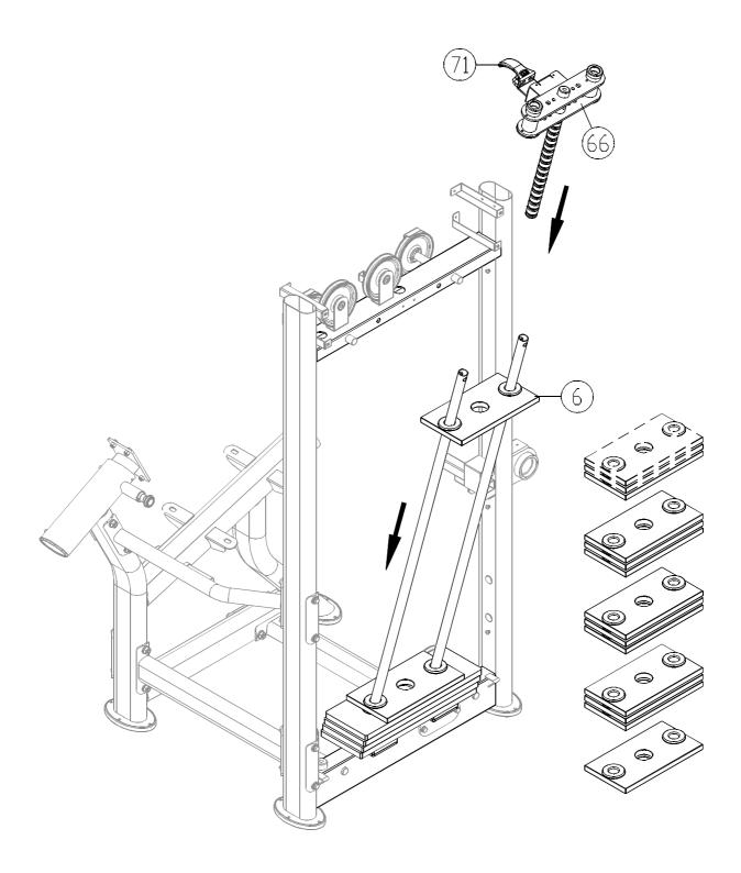
2-5. Insert and lower the 13 small (5 kg) weight plates (6) into place one at a time. **NOTE:** The convex side faces up.
