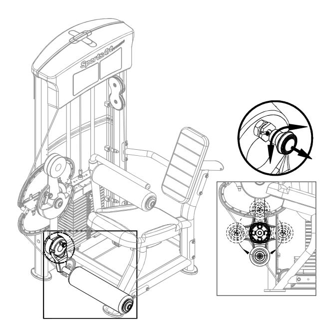
1-1. Pull out the knob to adjust the lower cushion arm position. You can rotate and secure the cushion arm for use within a 360 degree range. When released, the knob automatically engages to secure the position.
