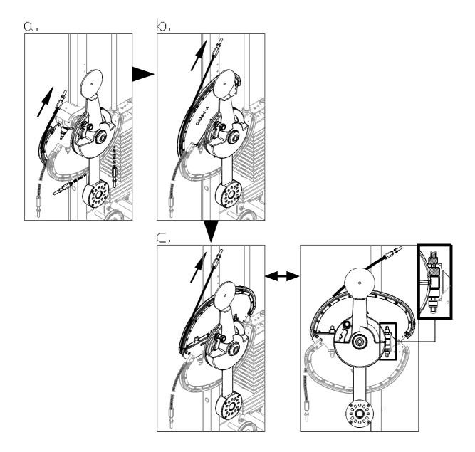
5-3. Follow illustrations to (a) feed the upper cable onto the cam cable channel; (b) pull the cable upward until the stopper rests on top of the tube.NOTE: The CAM arm rotates.
