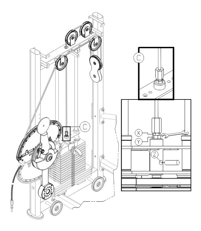
5-5. First insert an open end wrench into (Z) hole. Adjust the large nut at area C to the lowest position. Then, secure nuts (X,Y).
