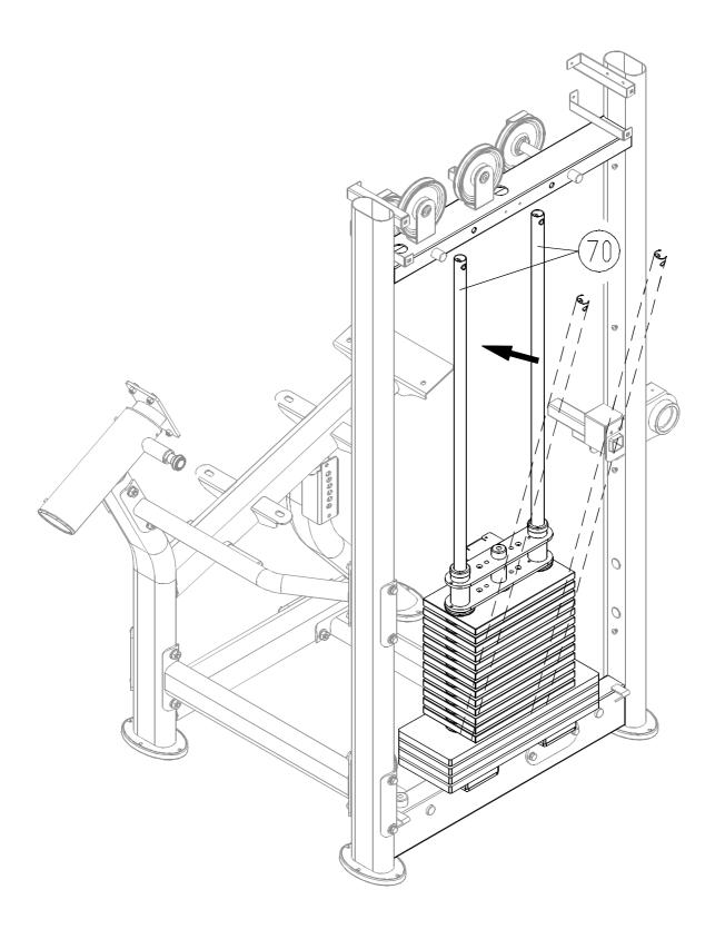
2-7. Tilt the guide rods (70) back into place.
