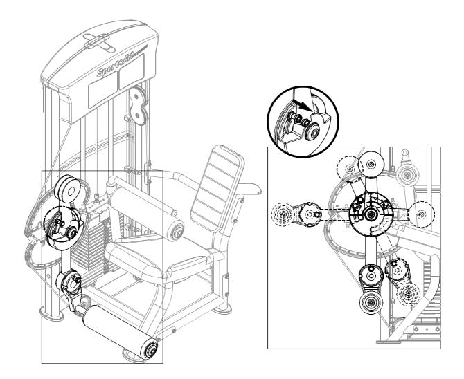
1-2. Pull out the knob on the rotator arm. Place the rotator as desired for use. When released, the knob automatically engages to secure the position.
