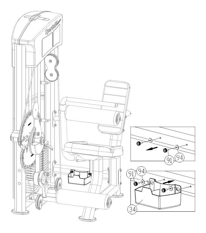
14-1. Before installing the bottle holder, remove hardware (91, 94) as shown.14-2. Hold the bottle holder in place (34) and secure it with hardware (91,94) as shown.
