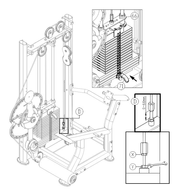
7-1. Insert the stack fork (71) into the gap under the lowest weight plate. Then adjust the large nut at area D. Adjust until the upper stack carriage set (66) moves slightly. To adjust the cable, first loosen (Y) nut. Then adjust (X) nut. If the cable is too long, adjust (X) nut downward. If too short, adjust (X) nut upward. After adjusting (X) nut, tighten (Y) nut against the weight stack to secure this position.
