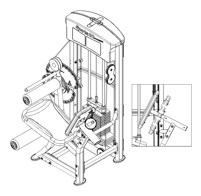
1-4. To move the seat back position toward yourself, simply pull it. To move the seat back away from yourself, pull the knob and press the seat back.
