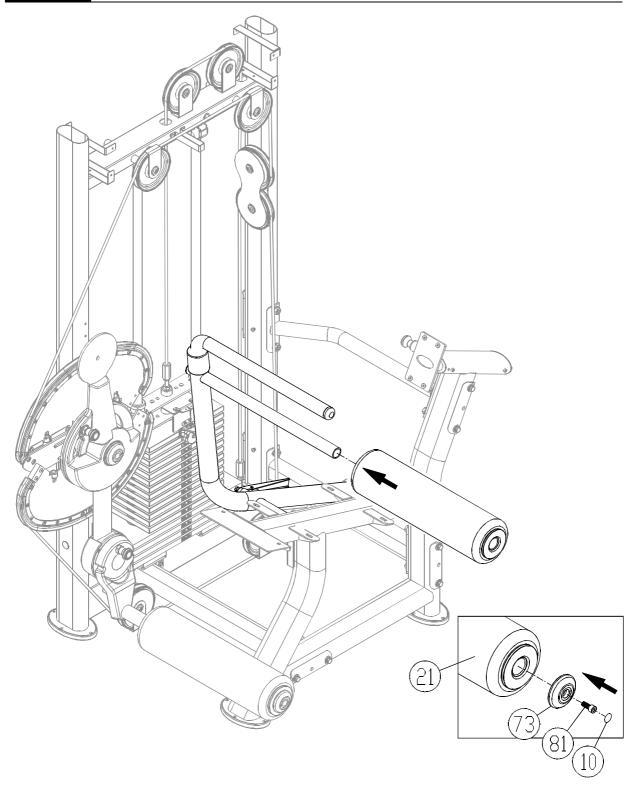
9-1. Put the cylindrical cushion (21) in place on the upper cushion arm. Then secure it with the cover (73) and screw (81). Then put the sticker (10) in place as shown.
