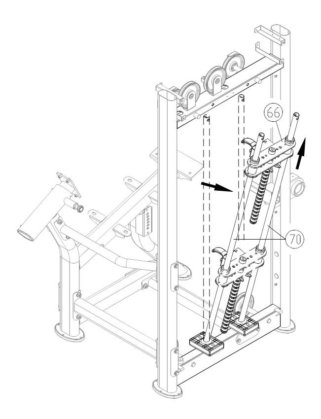
2-3. Tilt the guide rods (70) backward. Then lift the upper stack carriage (66) off the guide rods as shown. Carefully set the upper stack carriage aside.
