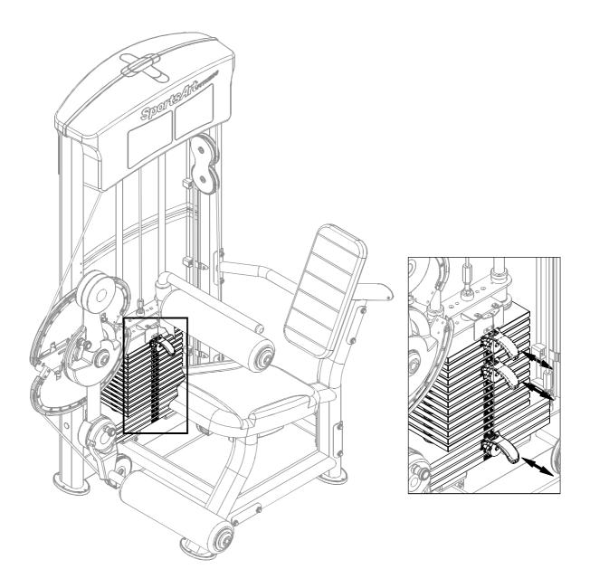
16-1. Insert the stack fork to make sure that every weight plate can be engaged easily.
