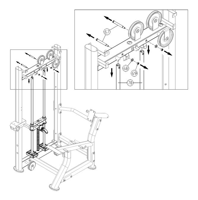
2-2. Remove hardware (67, 68, and 69). Guide the guide rods (70) downward as shown.
