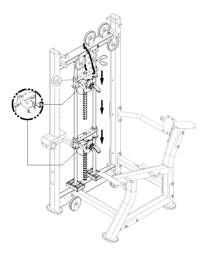
2-1. Hold upper stack carriage set (66) and cut the zip tie. Gently lower the upper stack carriage set (66) into place as shown.
