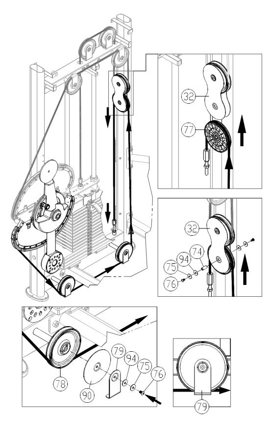
5-6. Insert the lower cable as indicated by the arrows, first feeding it into the lower channel of pulley B (78). Secure pulley B (78) with covers and hardware (90,79,75, 76,94). Continue threading the cable to incorporate other pulleys. Route the cable through the top side of the lower pulley A (77). Then secure that pulley wheel with hardware (74,75,76,94). Finally, secure the cable to the lower stack plate as shown.
